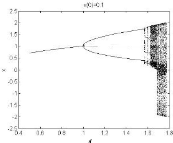
Fig. 4 Bifurcation diagram for the long term values of the system output  $x$  versus the parameter  $d$
