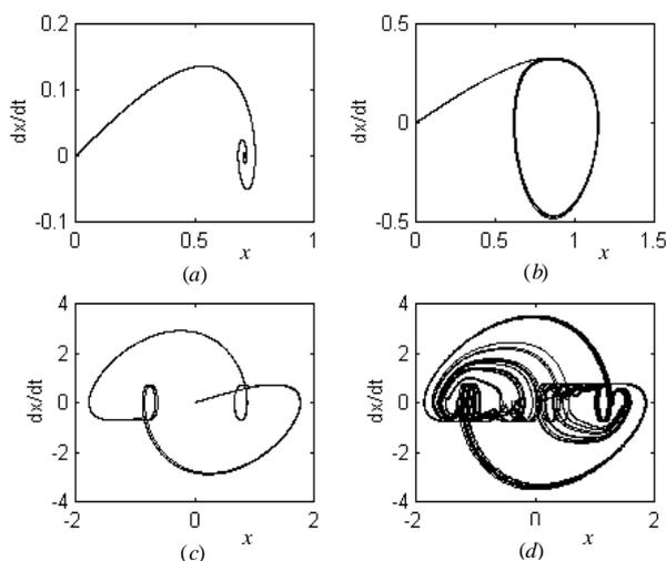
Fig. 2 Phase portrait of the system with  $\tau=\varepsilon=1$ : (a) for  $d=0.5$ , the system trajectory converges to the equilibrium point; (b) self-sustained oscillation for  $d=0.9$ ; (c) oscillations for  $d=1.51$ ; (d) chaotic behaviour for  $d=1.7$
