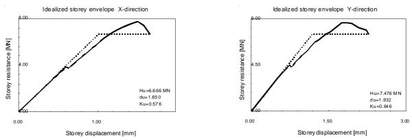
Fig. 6 Relationship between the resistance and relative storey drift of the storey for western wing for X and Y direction
