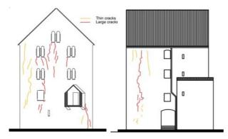
Fig. 8 Crack pattern investigation of the Pišece Castle (courtesy of Politecnico di Milano)
