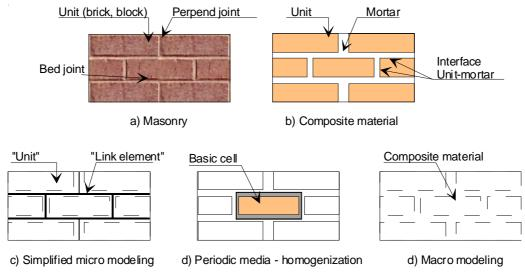
Fig. 3 Different levels of modelling brickwork masonry (after [6])
