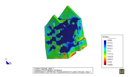
Fig. 12 PS1 model: Seismic analysis for the 1st modal shape – results for main tensile stresses
