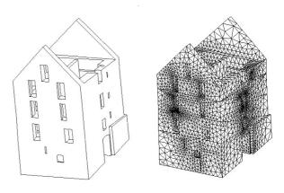
Fig. 9 P-model: geometry and mesh idealisation
