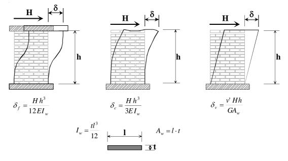
Fig. 1. Elastic deflections of masonry walls
