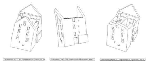
Fig. 11 1st, 2nd and 3rd modal shape for model PS
