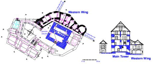
Fig. 5 Structural layout and cross-section of western wing and the main tower of the Pišece Castle
