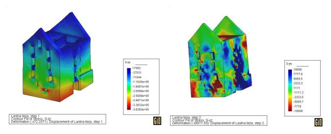
Fig. 10 Distribution of stresses [N/m<sup>2</sup>]: (a) normal stresses for model P under PG load case; (b) shear stresses for model H under load case HSS
