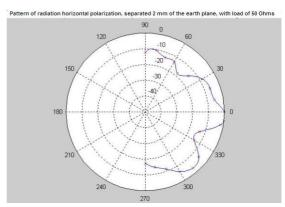
Fig. 12 Dielectric air, separation 2 mm,  $\phi$ =90°
