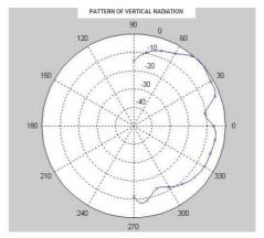
Fig. 13 Dielectric duroid, separation 3.6 mm,  $\phi$ =0°
