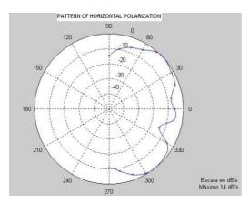
Fig. 14 Dielectric duroid, separation 3.6 mm,  $\phi$ =90°
