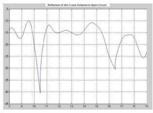
Fig. 4 Reflection in open circuit
