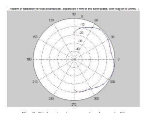
Fig. 9 Dielectric air, separation 4 mm,  $\phi$ =0°
