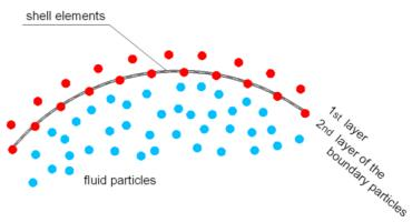
Fig. 5 Virtual fluid particles on the interface
