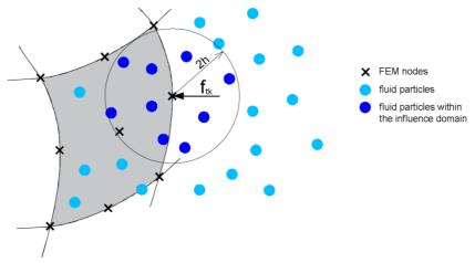
Fig. 4 Fluid forces on the structure
