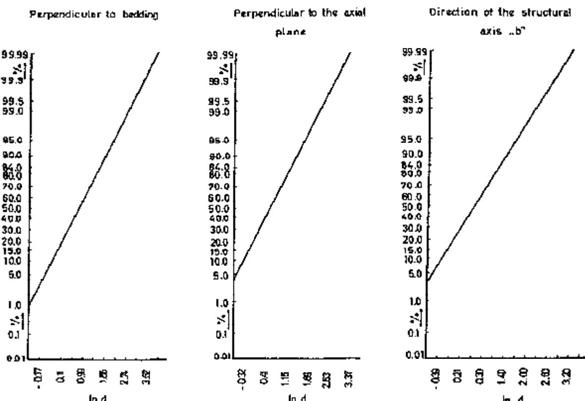
Fig. 1 Diagrams of cumulative frequency of measuring rock particle sizes
