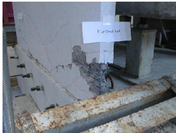
Fig. 9 Evolution of the cracking of the specimen's walls
