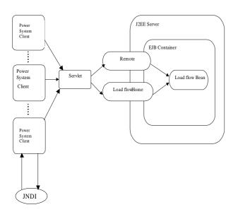
Fig. 1 Component model for Load flow Monitoring
