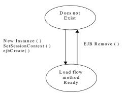
Fig. 3 Life cycle of EJB load flow Bean
