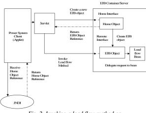
Fig. 2 Invoking a load flow method on the remote EJB Server
