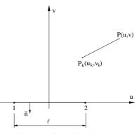
Fig. 2 Linear boundary element in the local co-ordinate system
