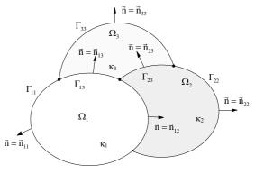
Fig. 1 Heterogeneous domain divided into three homogeneous sub-domains
