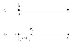
Fig. 3 Location of the collocation point  $P_k$  joined to the k-th node
