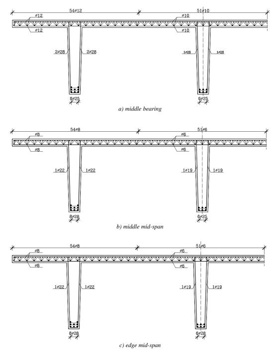
Fig. 4. Reinforcement of the main girders in characteristic cross-sections
