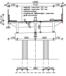
Fig. 2 Highway overpass - cross-section
