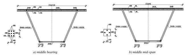
Fig. 11 Box girder reinforcement in characteristic cross-sections of the bridge
