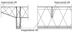
Fig. 15 Setting of longitudinal and transversal trusses
