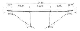
Fig. 7 Box girder bridge: longitudinal section
