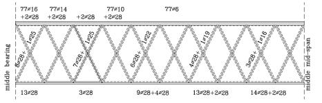
Fig. 10 Longitudinal disposition of the web reinforcement
