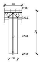
b) Cross-section reinforcement at the bearing
