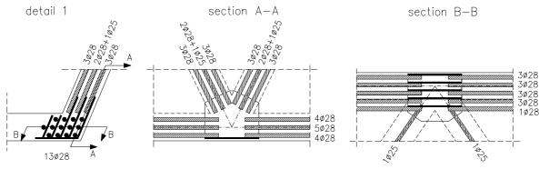
Fig. 12 Steel plates for reinforcement connection
