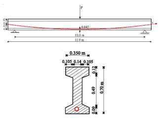
Fig. 5 Geometry of the analyzed I-beam
