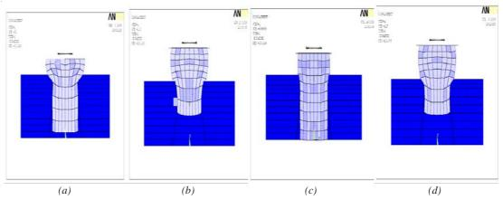
Fig. 7 The grid deformations at extrusion strain of 0.21 for die angles of (a) 12°, (b) 15°, (c) 25° and (d) 30°
