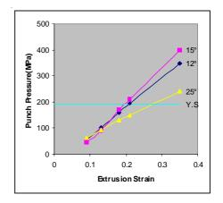
Fig. 10 Variation of experimental punch pressure with extrusion strain
