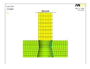
Fig. 3 Meshed model with degrees of freedom constraints
