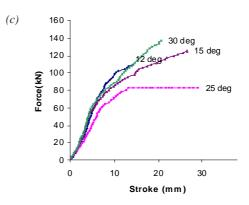
Fig. 9 Force – Stroke diagram for open die extrusion at (a) 0.09 strain, (b) 0.13 strain and (c) 0.21 strain
