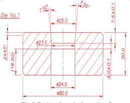
Fig. 8 Design of a typical extrusion die
