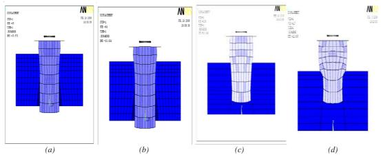
Fig. 6 The grid deformations at extrusion strain of 0.18 for die angles of (a) 12°, (b) 15°, (c) 25° and (d) 30°
