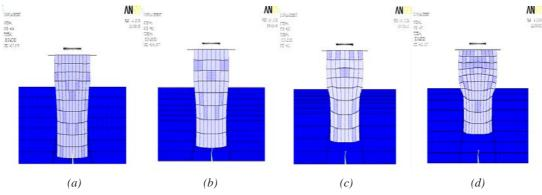
Fig. 5 The grid deformations at extrusion strain of 0.13 for die angles of (a) 12°, (b) 15°, (c) 25° and (d) 30°
