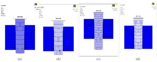
Fig. 4 The grid deformations at extrusion strain of 0.09 for die angles of (a) 12°, (b) 15°, (c) 25° and (d) 30°
