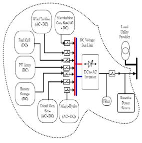
Fig. 8 Direct and centralized alternating current based MG architecture [9]
