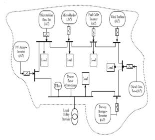
Fig. 7 Alternating current based MG architecture [9]
