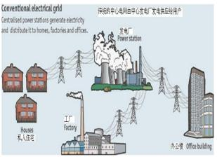
Fig. 5 Conventional power grid configuration [8]
