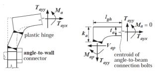
Fig. 1 Deformed shape and body diagram of the angle
