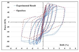
Fig. 3 Calibration of the reference bridge pier
