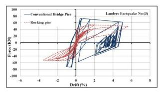
Fig. 8 Hysteretic behaviour results of conventional and rocking pier in Landers records
