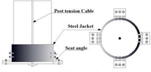
Fig. 4 Scheme of the proposed rocking pier
