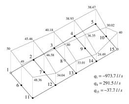
Fig. 8 Computed hydraulic heads and reservoir flows values
