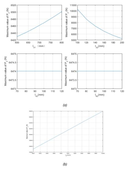
**Fig. 9** *Driving force curve of cylinder influenced by component size*
