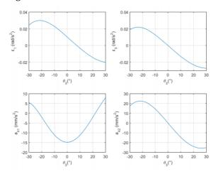
Fig. 6 Angular acceleration of the actuator and acceleration curve of the centroid
