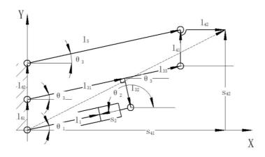
Fig. 3 Motion vector diagram of the mechanism
