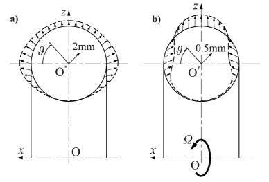
**Fig. 4** Toroidal shell cross-section deformation due to a) internal pressure and b) centrifugal load, [33], (with indicated scale)
