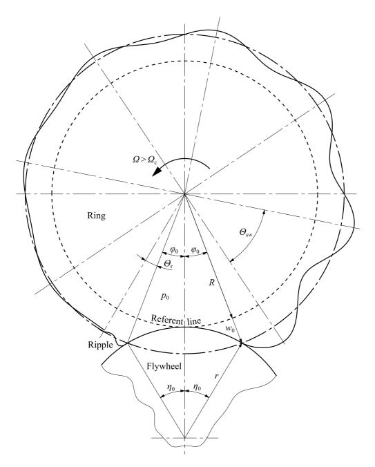
**Fig. 9** Ring standing waves and ripple,  $\Omega_c = 320$  rad/s,  $\Omega = 400$  rad/s
