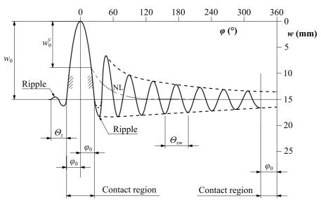
Fig. 19 Calculated ring standing waves, boundary conditions according to experimental results,  $\Omega = 400 \text{ rad/s}$
