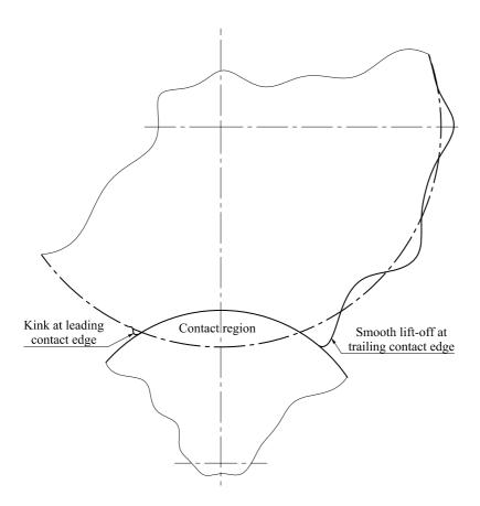
**Fig. 14** Lower portion of the balloon profile extracted from video data,  $\Omega = 420$  rad/s = 67 Hz, according to [7]
