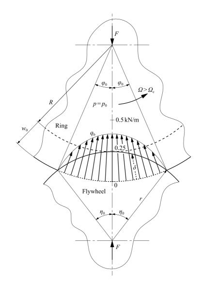
**Fig. 10** Radial internal load due to flywheel penetration in the rotating ring,  $\Omega = 400$  rad/s
