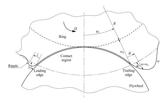
Fig. 6 Boundary conditions at contact edges
