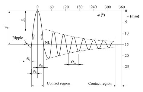
**Fig. 13** Calculated ring standing waves,  $\Omega = 400 \text{ rad/s} = 63.7 \text{ Hz}$
