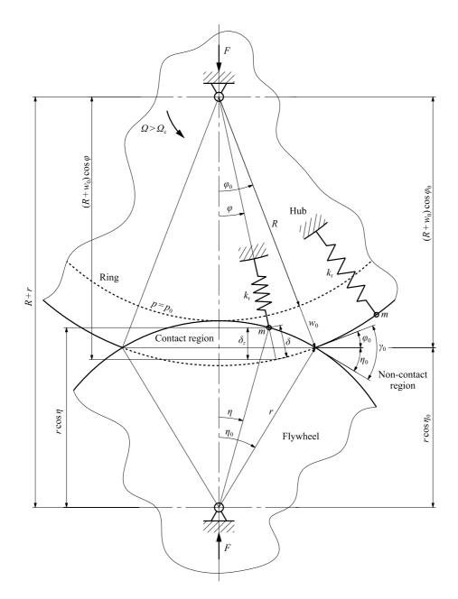
Fig. 7 Determination of edge discontinuity angle,  $\gamma_0$ , and bearing reaction forces, F
