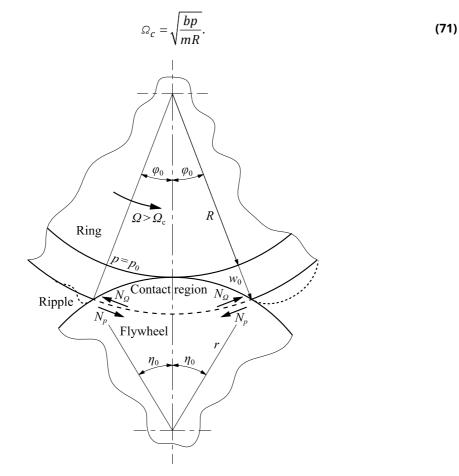
**Fig. 8** Moving-mass-induced membrane force,  $N_{\Omega}$ , and inflation pressure membrane force,  $N_{p}$ , and generation of standing waves
