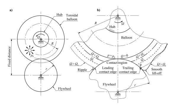
Fig. 1 Experimental set-up and balloon deformation (according to [7])
