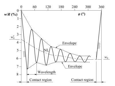
**Fig. 11** Recorded standing waves of a balloon tyre,  $\Omega = 420$  rad/s = 67 Hz, according to [7]
