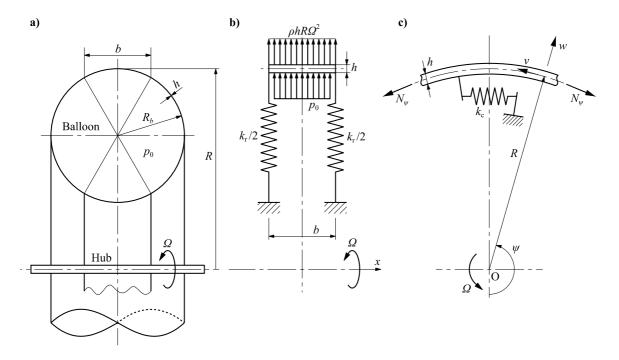
Fig. 3 Toroidal balloon and the corresponding ring model
