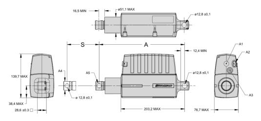
Fig. 12 Scheme of Electrak Pro actuator [15]
