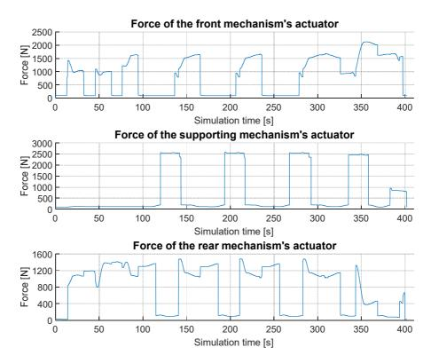
Fig. 9 Load variations in the actuators of wheelchair lifting mechanism drive
