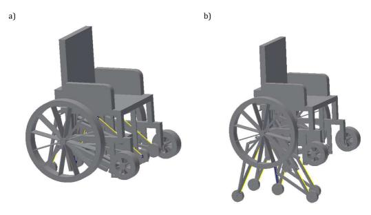
Fig. 16 A side model of the wheelchair with the mechanisms: a) folded, b) spread out
