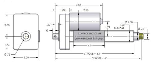
Fig. 11 Scheme of TMD02 actuator. Dimensions in inches [14]
