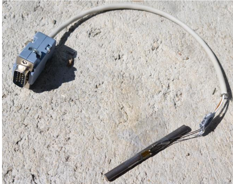
Figure 47. Strain gauge on a prestressing steel sample used for temperature compensation
