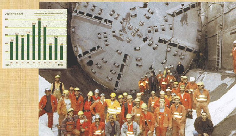
Design of the machine Hard Rock single shield machine
