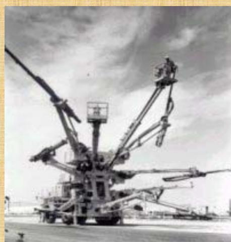
The first seven-arm drilling jumbo
